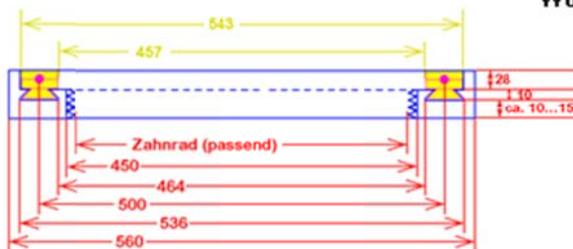
In the top part of figure 5, we see the Top-view, and in the bottom part of figure 5 we see the side-view of the rotation ring, carrying many magnets. The magnet-carriers, as we know them from figure 4, are drawn in yellow colour. Their position and their orientation can be arranged in figure 4, and they are fixed with stable (for instance M12-) screws as mentioned above.
