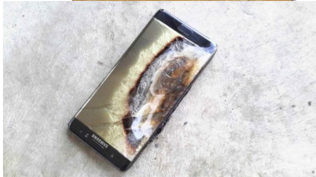
Failure Samsung Galaxy Note 7 2016
